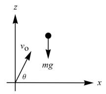
Newton's second law states that the sum of the forces on the ball is equal to its mass times acceleration.
